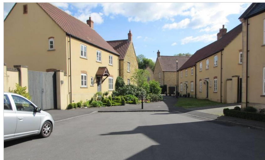
Where cul-de-sacs are unavoidable, they should be designed as informal public spaces with clear, direct and well overlooked pedestrian connections.
